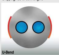
Material: HDPE - 80 (1.25") Grout Volume per 100ft: (1.0 TC) 125gal Fluid Volume per 100ft = 15gal Shipping: 200-500ft coils
